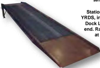
Stationary ramps, series YRDS, include an Edge-Of-Dock Leveler at the truck end. Ramp height is fixed at 50". Leveler offers service range of +/- 5".
